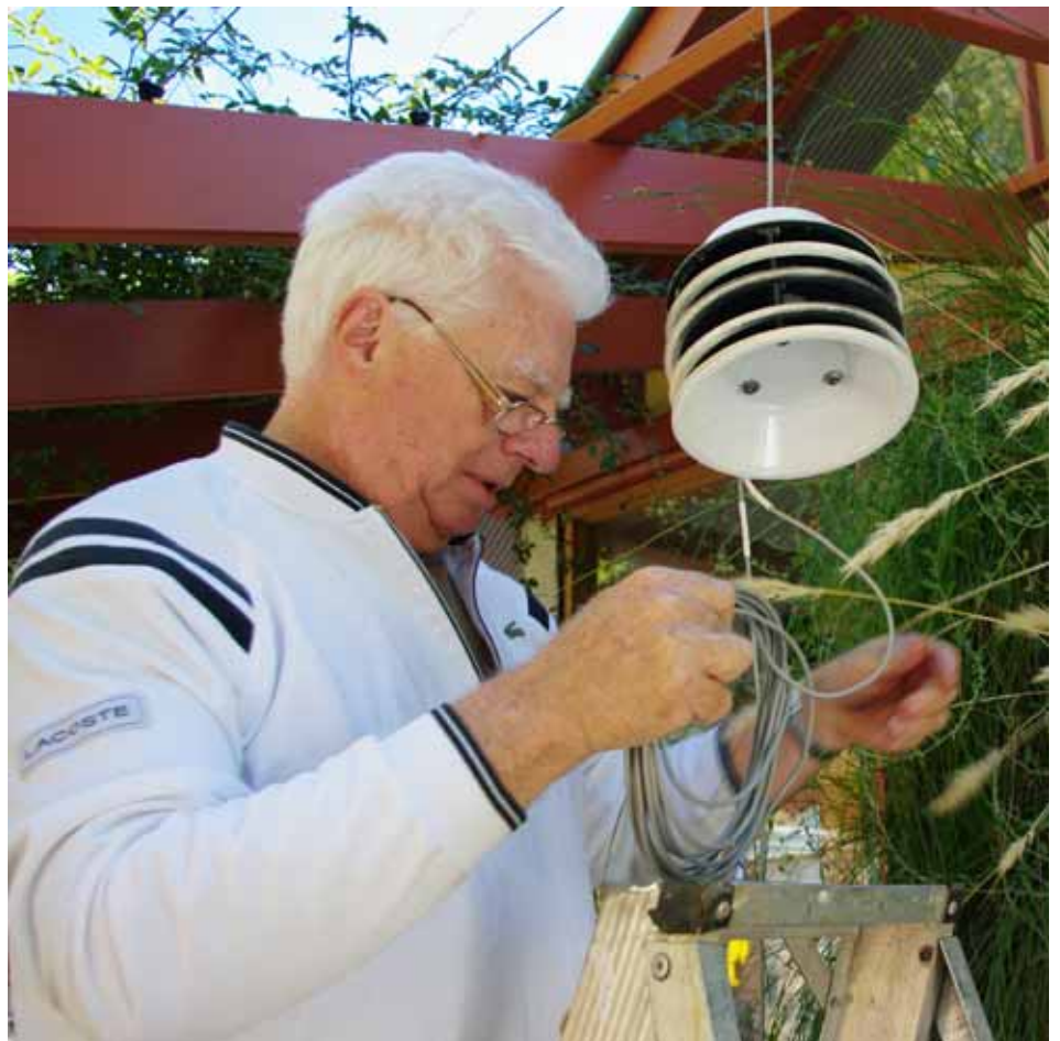
University of Adelaide Associate Professor Terry Williamson installing temperature loggers on Fifth Creek Studio's trial living walls in 2009 (Photo sourced from Fifth Creek Studio)
